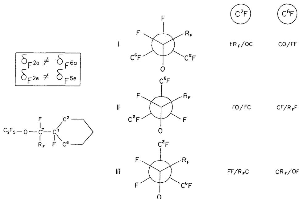
Fig. 1. Newman projections along the C(1)–C(7) bond of compounds **5** ( $R_F = CF_3$ ) and **6** ( $R_F = C_2F_5$ ).
